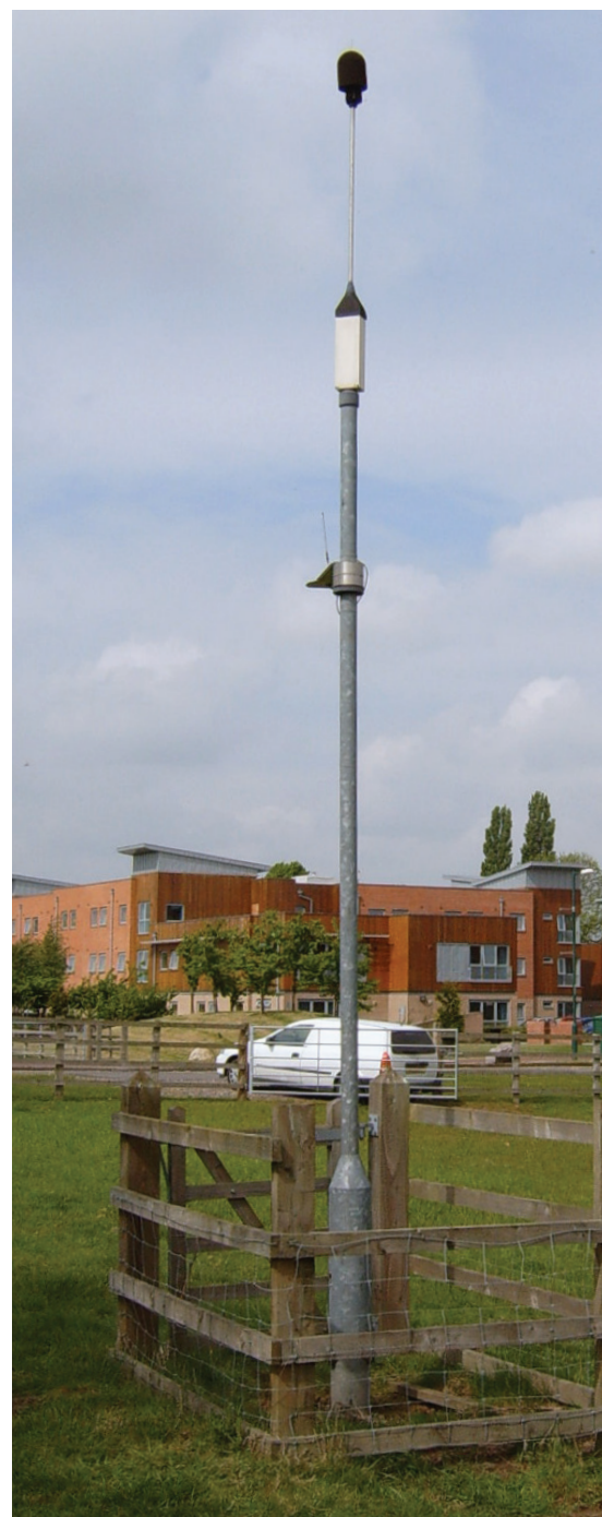
CR:243/4 "Noise Pole" installed as 1 of 7 monitors in an airport noise monitoring system
