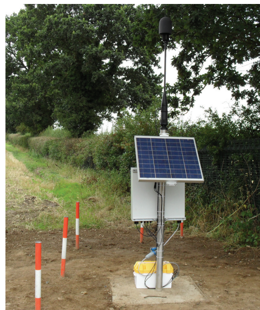
CR:243/1 Noise Monitor installed to measure noise from aircraft engine testing
