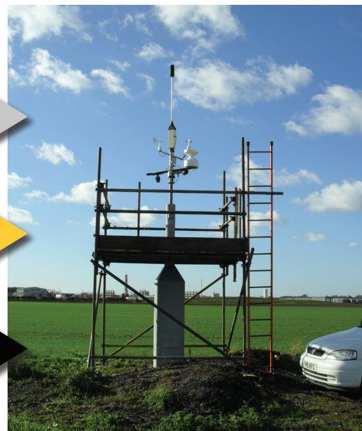
CR:243/1 Noise Monitor during annual calibration and servicing
